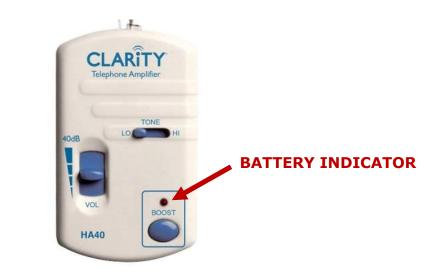
When the battery is drained, if the volume level is moved to the lowest (down) position, the handset will work. When the volume level is at any other position, the handset WILL NOT operate.
